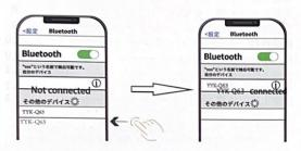
As soon as the earphones are placed in the charging case, they turn off. It will then begin charging. Once the earbuds are removed from the case, they will immediately turn on and automatically pair and connect to a paired Bluetooth device.
